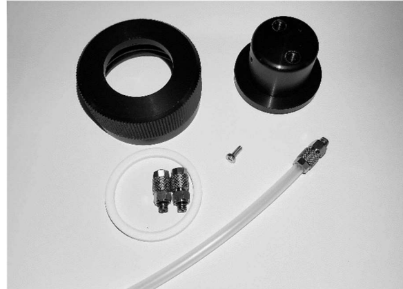
Step 4: Clean aluminum inner and outer cap parts with acetone, reassemble by reversing steps.
