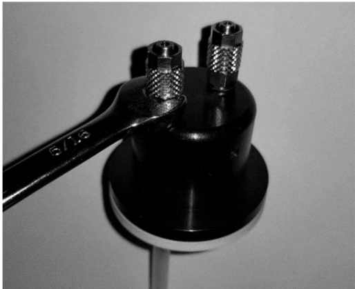
Step 3: Use a 5/16" wrench to remove all three ink line adapters. Use caution not to over tighten on reassembly. Be sure that o-ring is in place around base of adapter.
